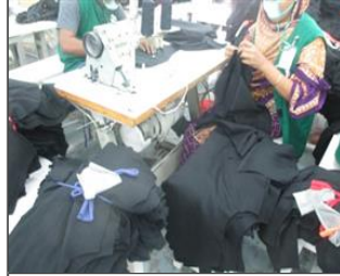
Photo of non-conformity Sewing operator was seating very close to pulley cover which may arise vulnerable risk.JPG
